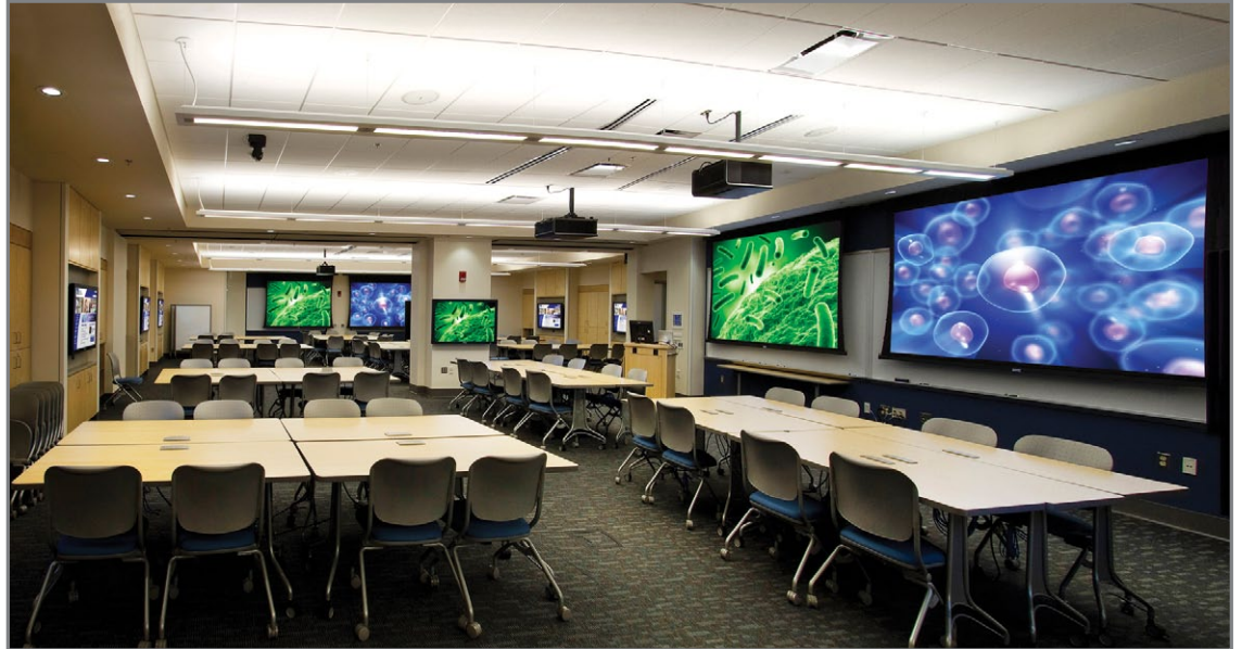
The Integrated Teaching and Learning Center at the University of Massachusetts Medical School features one 55-inch LCD display per student work group, and side-by-side projection systems (two projectors per classroom section).
