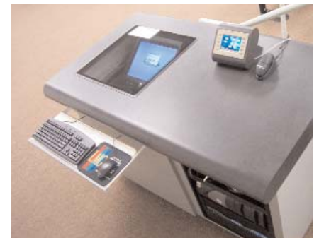
Teaching consoles like this one are in all 18 of the new rooms, featuring such components as a Crestron touchpanel, wireless mouse and built-in monitors, keyboard and equipment rack.
