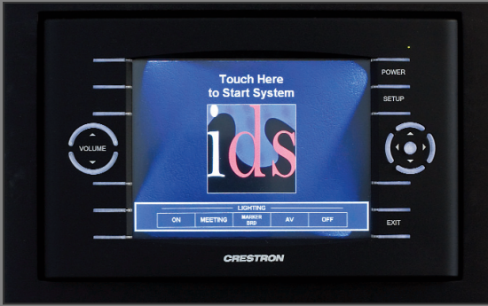
Crestron TPS-6X touchpanel wall mounted at IDS. The touchpanel releases from the docking station and used wirelessly anywhere in the room.
