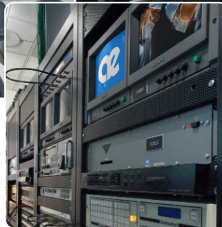
An Aethra videoconferencing system makes it possible to share the learning experience across great distances. A single operator in the OLC's control room can monitor video and computer feeds, audio, switching, digital recording and playback
