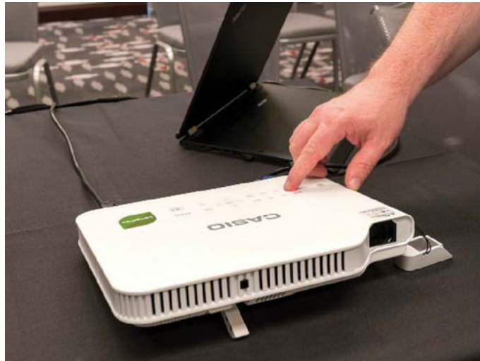
This new line of LampFree projectors use a hybrid LED and laser light source instead of a projection lamp.
